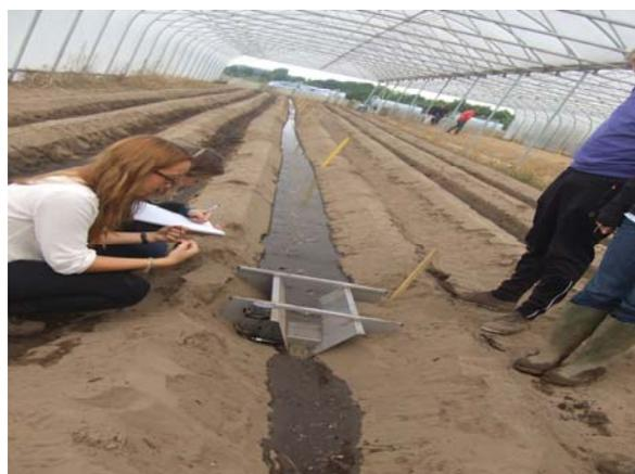
The practical of infiltration measurement in Alterra.
